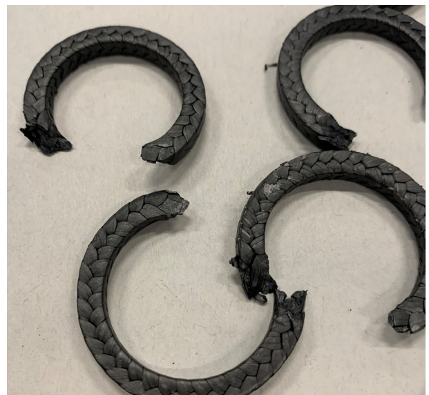
Braided packing cut into rings with frayed ends
