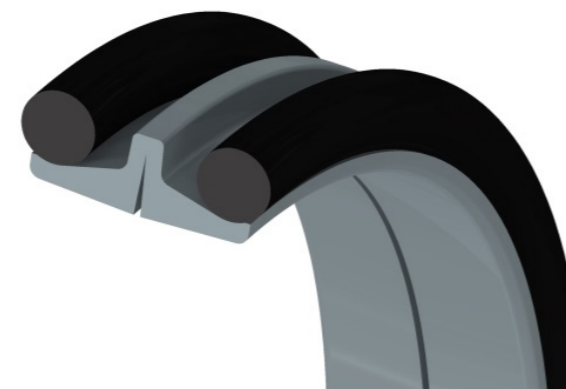
Render of a driveline mechanical face seal
